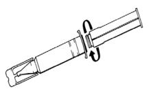
3. Twist the protective tab and then, without bending, pull slightly to break the seal.
