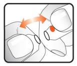
The ampoule can only be broken in one direction. The breaking point can be found on the neck of the ampoule next to the red dot. The pressure must be applied under the red dot.
