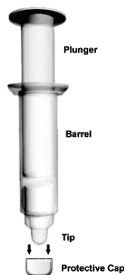
Fig. 1: Diagram of dispenser
