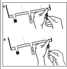
• Immediately before inserting the infusion set, break off the tamper evident arrow flag from the blue infusion port (A).
