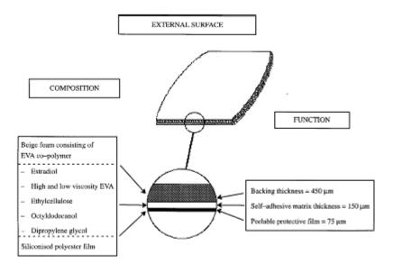
OESCLIM® patches are made up of a self-adhesive polymer matrix, which contains the estradiol, backed onto a rectangular foam mounting with rounded corners. The adhesive surface is covered by a transparent silicone-treated protective film which must be removed before use. This system provides excellent local tolerability and adhesion.
