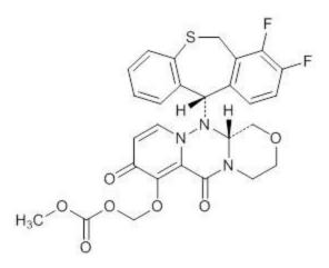
Physicochemical properties: White to light yellow powder. Practically insoluble in water at 25°C and fasted-state and fed-state simulated intestinal fluid.
