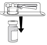
Remove the paper backing from the MIXJECT device. Do not remove the MIXJECT device from the blister pack. Place the vial on a hard surface. Center the MIXJECT device on the stopper and push straight down onto the vial top until it snaps securely into place. Remove the blister pack from the MIXJECT device.
