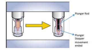
Remove autoinjector from the injection site, perpendicular to the skin. The protective shield automatically moves into place over the needle. The protective shield is then locked and the needle is protected.
